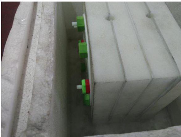
(a) Stator inside the Styrofoam box containing liquid nitrogen
