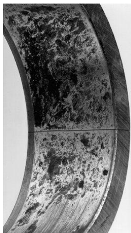
(a) Damaged bearing due to wear [11]
