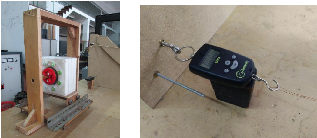
Figure 3.24: Experimental setup to measure guidance forces.
