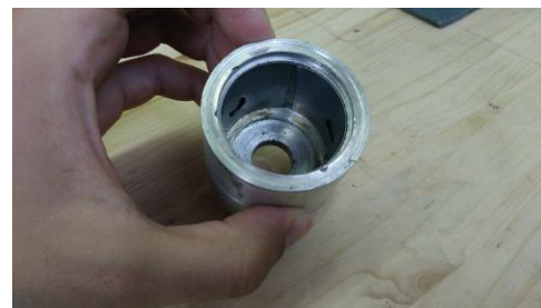
(b) Iron sheets placed inside the aluminium rotor
