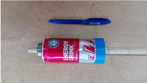
Figure 3.10: Rotor made from a can.
